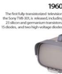
1960 The first fully transistorized television, the Sony TR-301A, released, including 23 silicon and germanium transistors, 15 diodes, and two high-voltage diodes.
