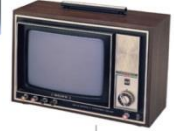
1970 Sony introduces Trinitron, its line of aperture grille cathode ray tube televisions, with the Sony KV-1320.
